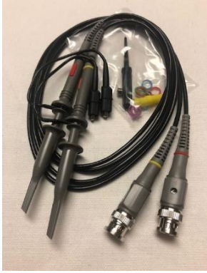
(2x) Oscilloscope Probes, spring loaded grabbers on left, BNC connector on right side. Only use these on an oscilloscope.
