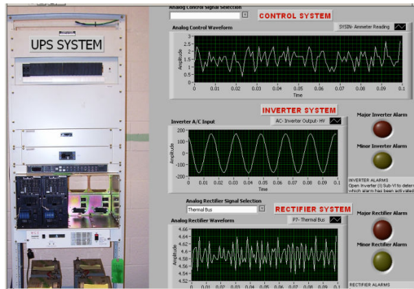
Fig. 3. Front Panel View of UPS Main Program Interface
