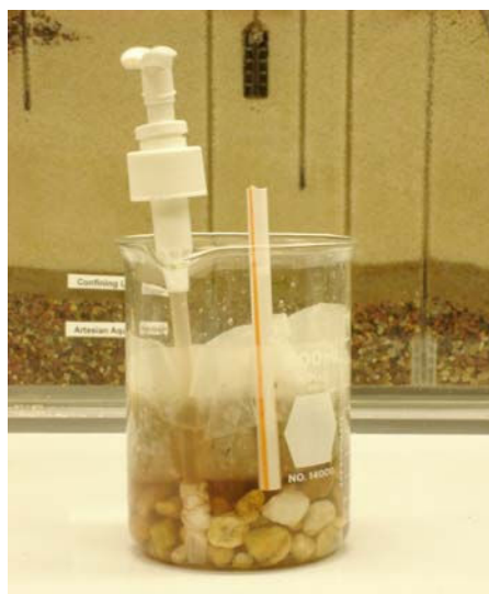
Figure 2. Aquifer model constructed by students for the groundwater remediation lab activity.
