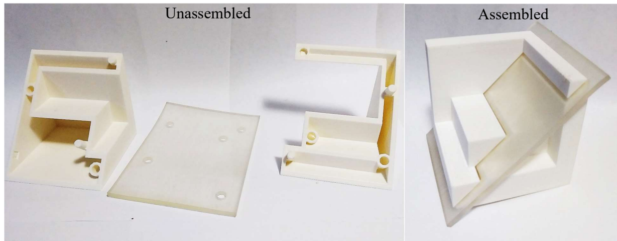
Figure 4. Photographs of three part 3-D printed TMCT Object before and after assembly.
