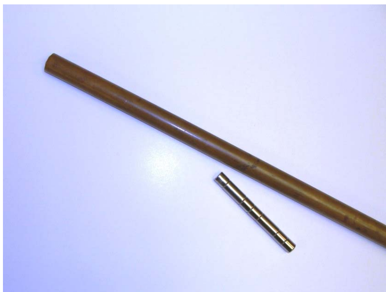
Figure 10: Magnet Falling in Copper Tube Apparatus.
