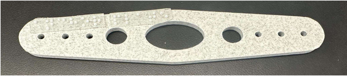
Figure 5: The anchor plate from Assignment 1 had a small fillet at the top and bottom edges of the perimeter, which were not noticeable to the student by touch.
