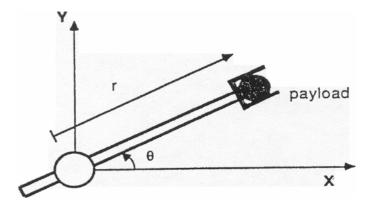
Figure 2. Two-joint Planar Robot
