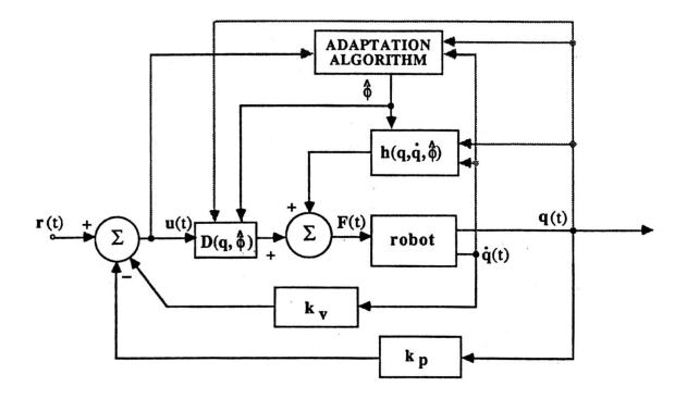
Figure 1. Adaptive Algorithm Block Diagram
