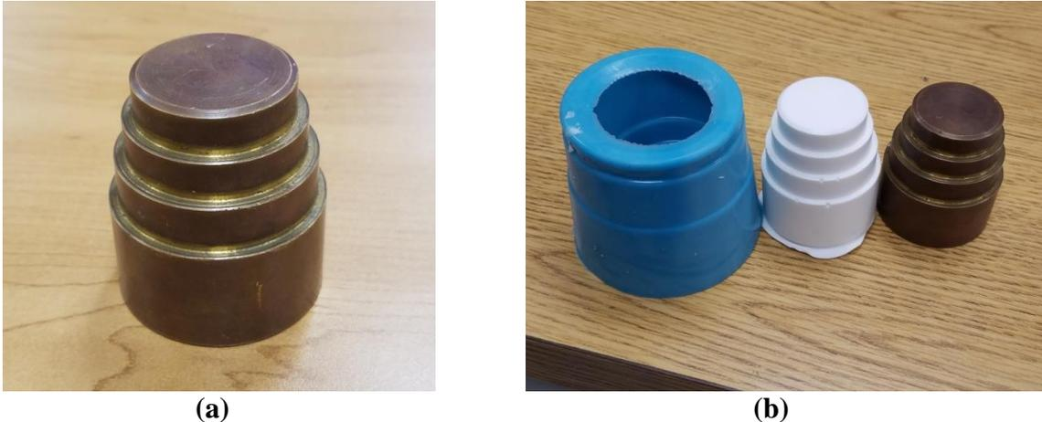
**Figure 4: a) Step mandrel; b) Silicone mold, cast part, step mandrel (from left to right)**
