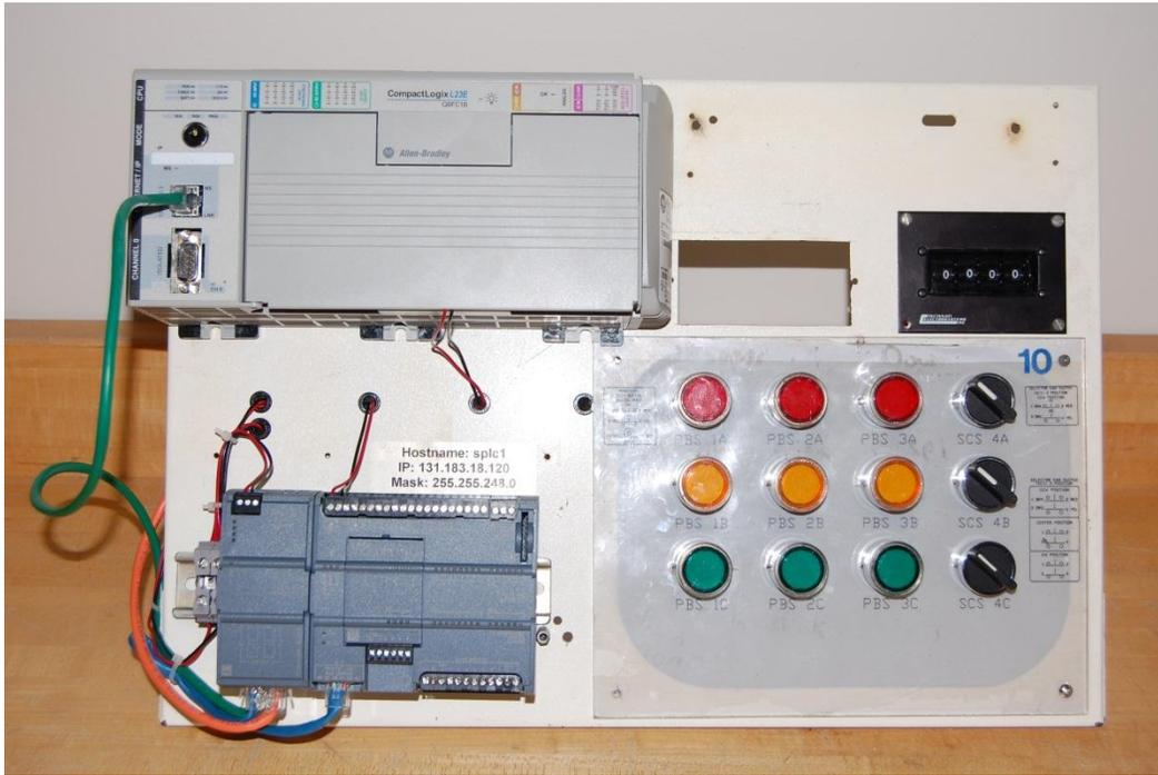
Pictured above are the two PLCs located on the trainer. On top is the A-B L23 processor. On the bottom is the Ethernet switch and Siemens' 1200 processor. Below is a picture of some students in the lab using the new trainer.
