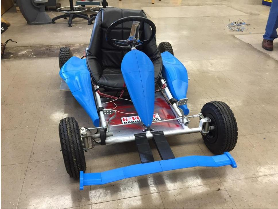
**Figure 7: Electric go-kart with 3D printed body parts**
