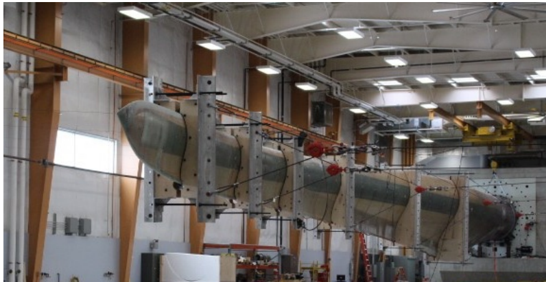
Figure 8. Strength testing of a 56-m long wind turbine blade
