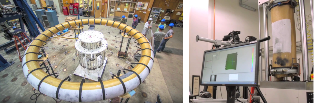
Figure 6. An inflated ring of HIAD being tested at UMaine's Advanced Structures and Composites Center
