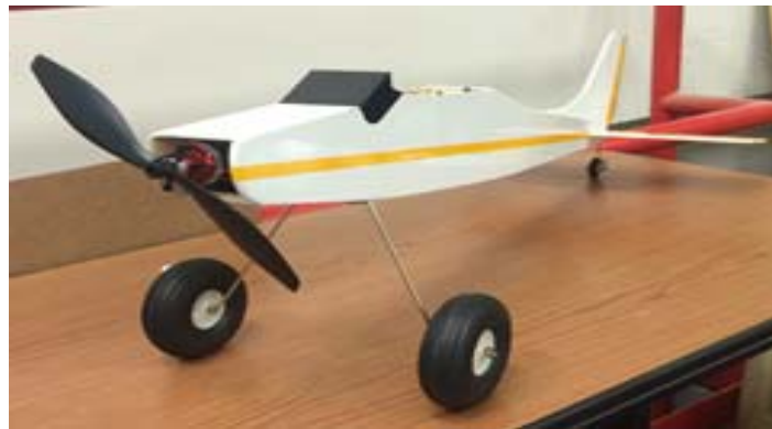
Figure 4. Construction in progress of balsa and monocoat high wing L19
