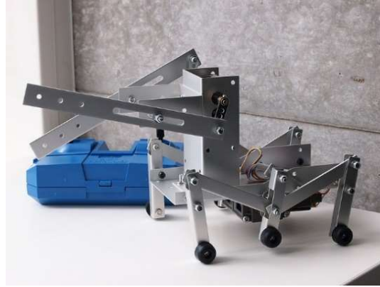
Figure 5-2: Assembled 6 legs boxer robot
