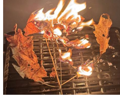
Fig. 6. Shows the dry maple leaves ignited and the embers sloping toward the wind direction and detected by the SEN55 that was placed in the left side of the setup. The dry leaves were placed on a non-combustible surface.
