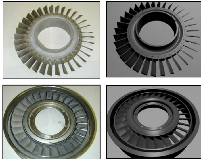
Figure 6: Engine blades modeled (right) from the actual engine (left)
