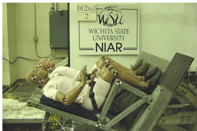
Figure 15. Pair of hybrid ii ATD's seated on two iron seats side by side
