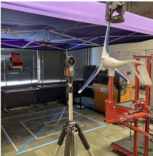
Figure 9: Anemometer and fan are aligned with the hub centerline.
