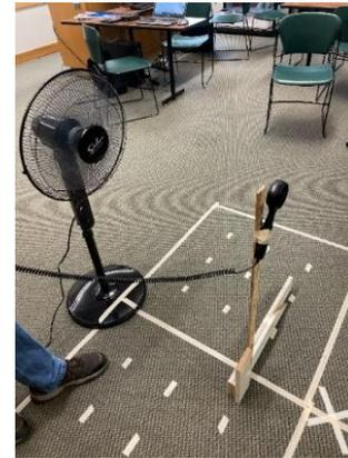
Figure 2: Rudimentary wooden block set up to hold the anemometer.
