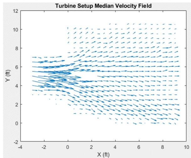
Figure 10: Velocity field showing the flow disturbance caused by the wind turbine.
