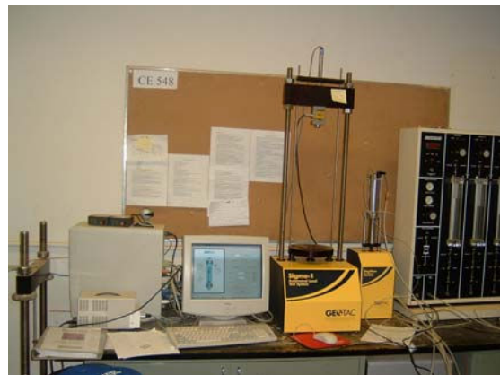
Figure 1. Set for Triaxial Experiment: a) Testing Chamber and b) Loading Frame
