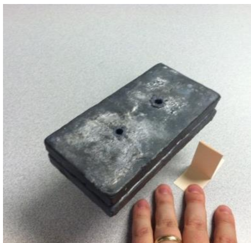
Fig. 3: Acceptance testing is performed by placing the masses on top of the widget and sliding a 1.75" spacer underneath.
