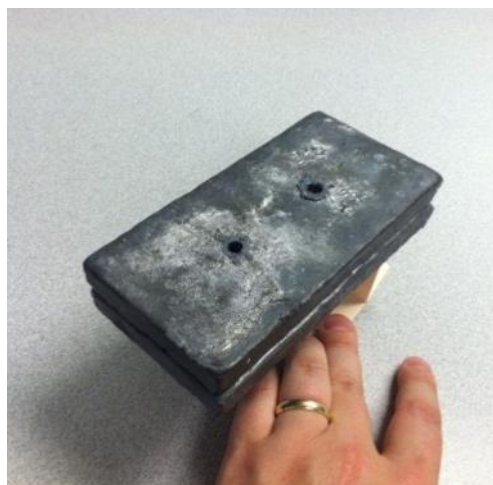
Fig. 3: Acceptance testing is performed by placing the masses on top of the widget and sliding a 1.75" spacer underneath.
