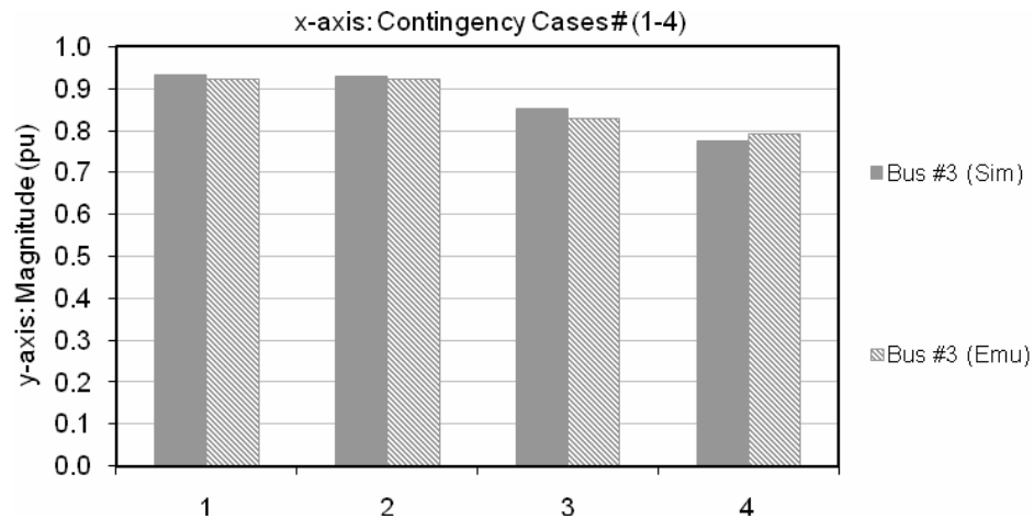
Figure 7: Comparison of Simulated (Solid) and Emulated (Striped) Contingency Results for Voltage Magnitude at Bus #3
