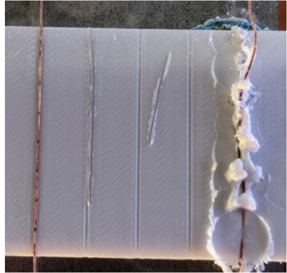
Figure 4 – Successful vs Failed Embed Events
