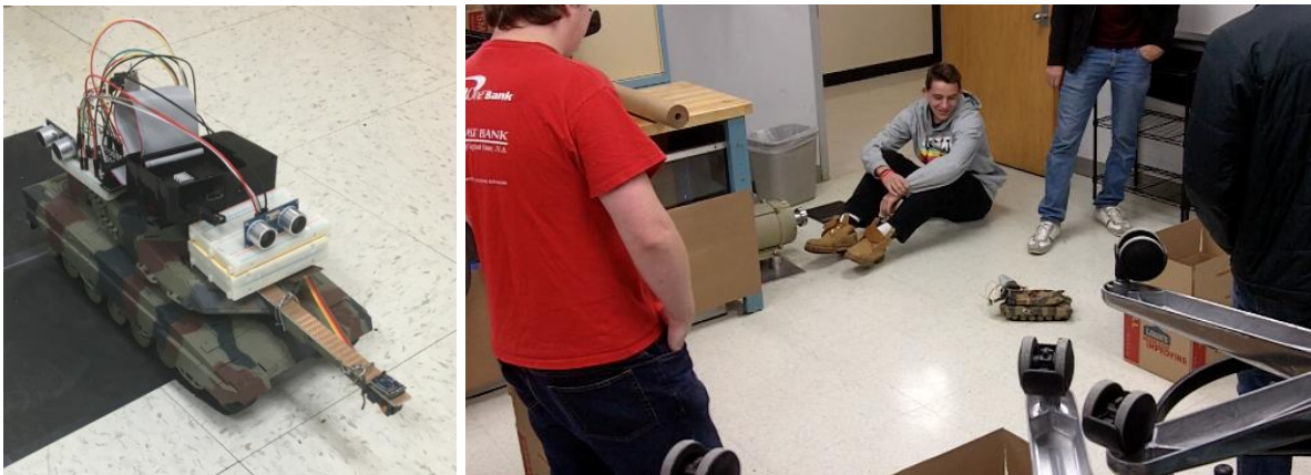
Figure 2: Raspberry Pi Tank (left) and student team conducting tank maze testing (right)
