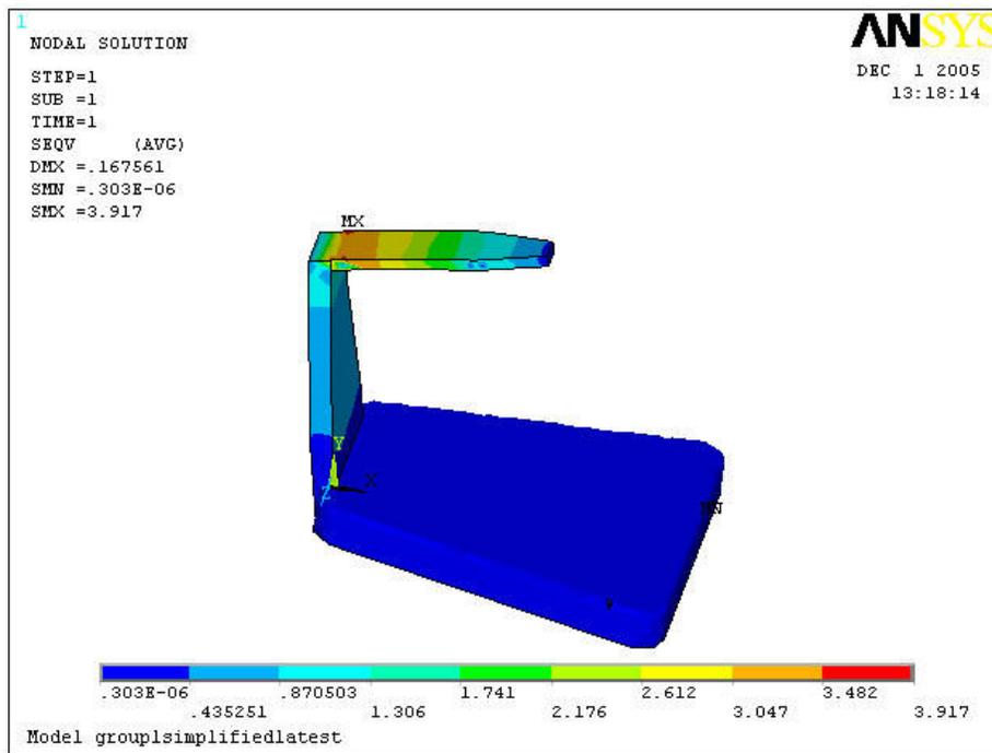
Figure 4. Team A's Simplified Banana Hanger: von Mises Stresses
