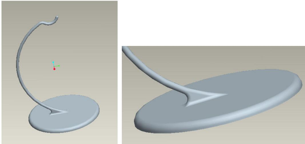
Figure 5. Team B's 'Banana Peg': 3D Model in Pro/Engineer
