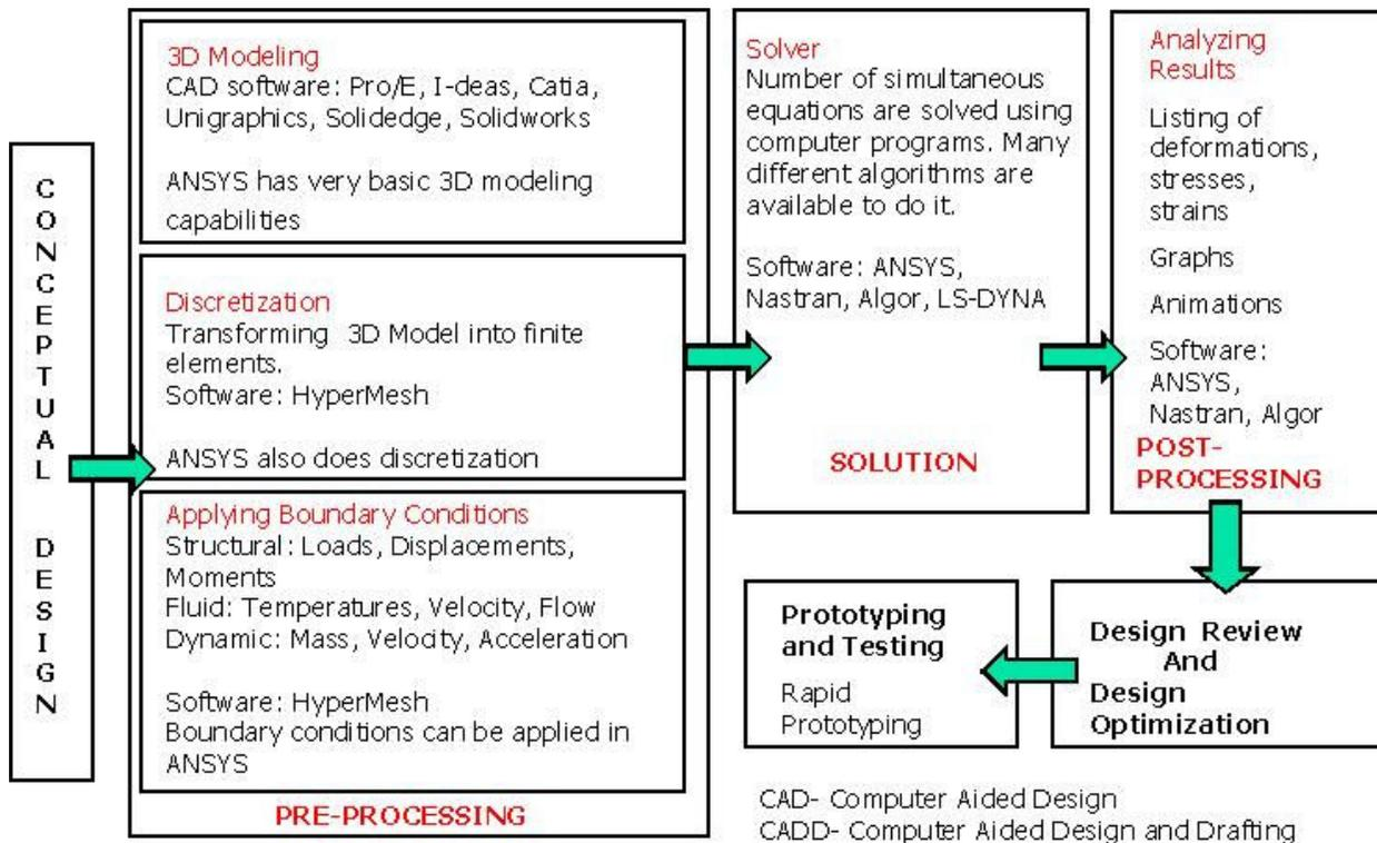
Figure 2. Stages in Computer Aided Engineering with Reference to Software
