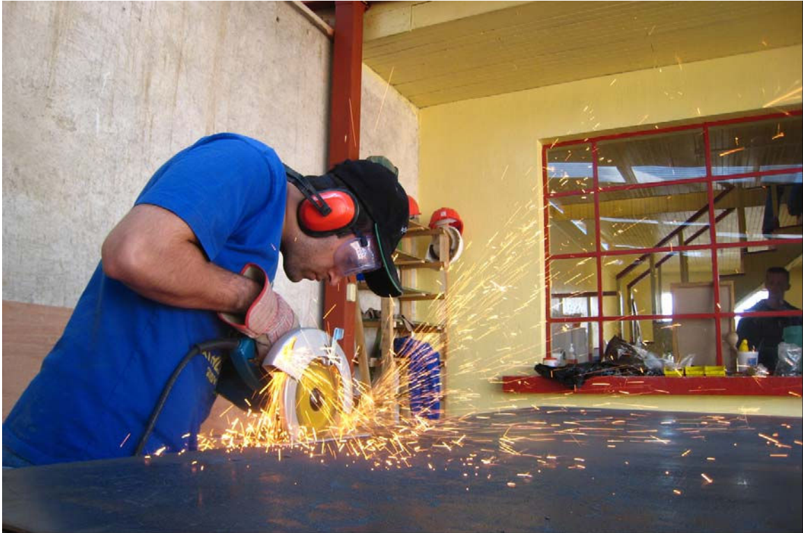
Figure 14 Using a Circular Saw to Cut Sheet Metal
