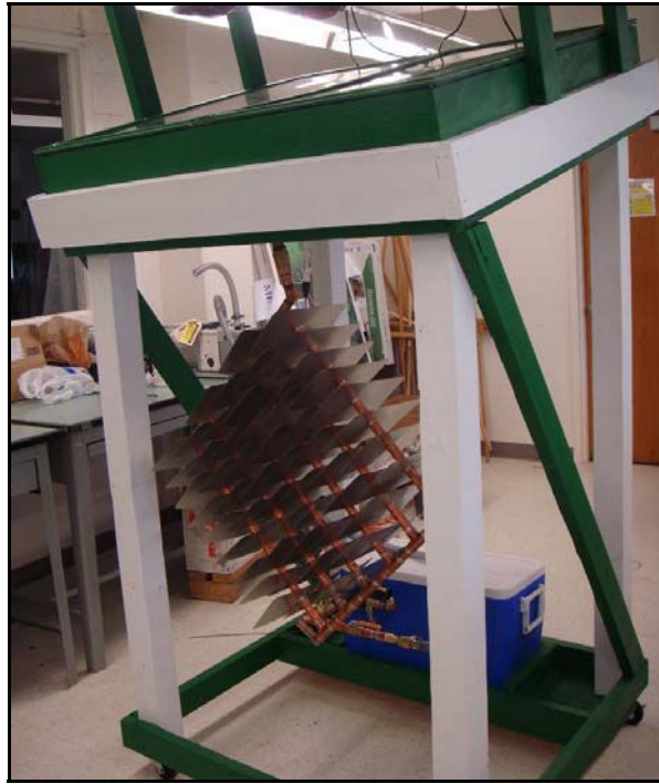
Figure 7. Completed assembly of adsorption refrigerator.
