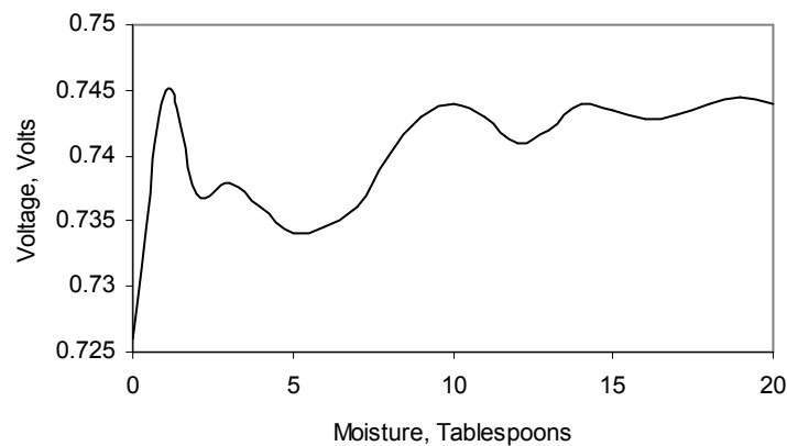
Figure 3. Moisture response of nails sensor
