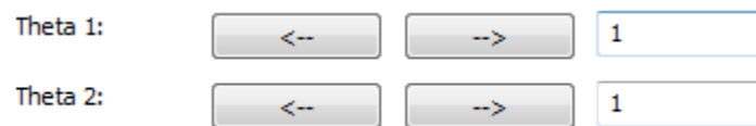
Figure 5: The buttons move each joint by the degrees specified in the box to the right.
