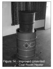
unhealthy and a fire hazard. An improved bucket burner has been developed; however, the improved model still produces so many harmful gases that the air quality is so toxic that researchers find it hard to understand how anyone survives the exposure. If the structure is improved to being less drafty burning coal in an unvented stove could be fatal. See Figure 14.
