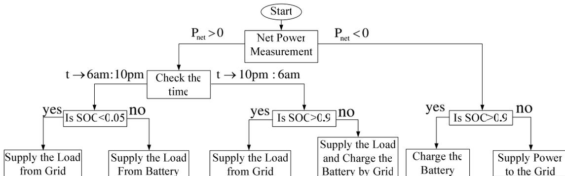
Fig.8. Operation mode controller for the proposed system.
