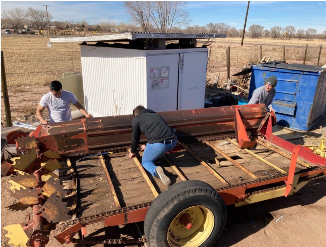
Figure 1: The trailer being converted to support solar panels for future on-the-go charging of equipment. One of the student groups worked on this community project.
