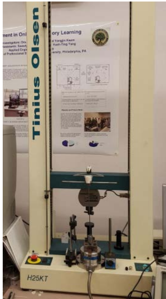
Figure 7: Stress testing of ultrasonic welded plastic parts.
