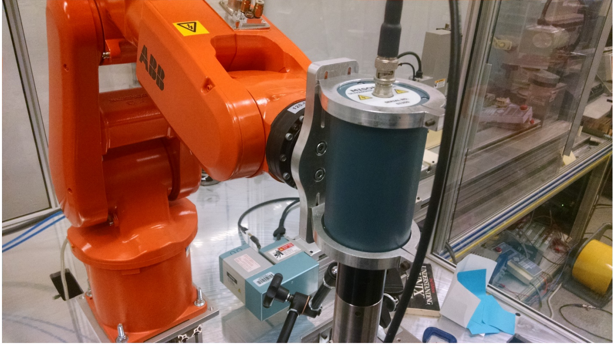
Figure 4c: Robotic Ultrasonic Welding System (with thermal camera and force sensor).
