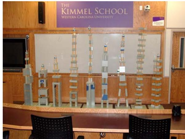
Figure 3 Nine towers were built by the American class. The tallest unit to pass earthquake test is fifth from the left. The tower voted overwhelmingly the most aesthetically pleasing was the last tower on the right.
