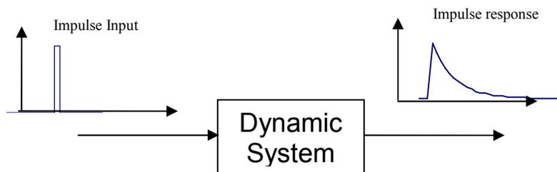
Figure 3: A dynamic system under Impulse input test
