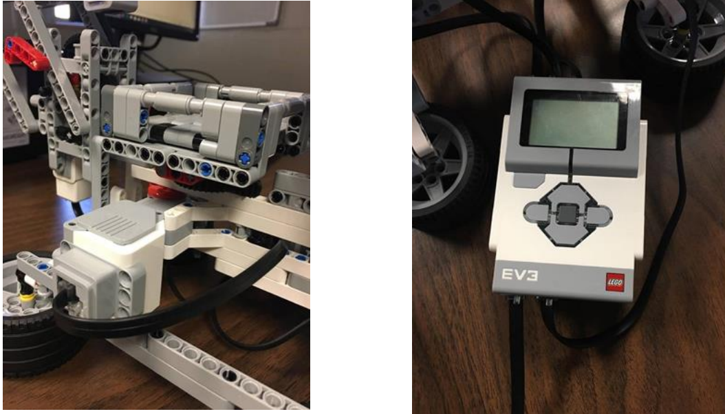
Figure 1 (a) Infrared sensor attached to an actuator to rotate a cube; (b) EV3 Mindstorms Brick (Controller)
