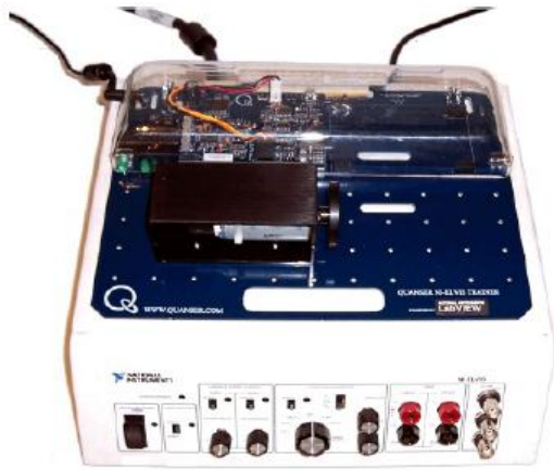
Fig. 2. DC motor system on the Elvis
