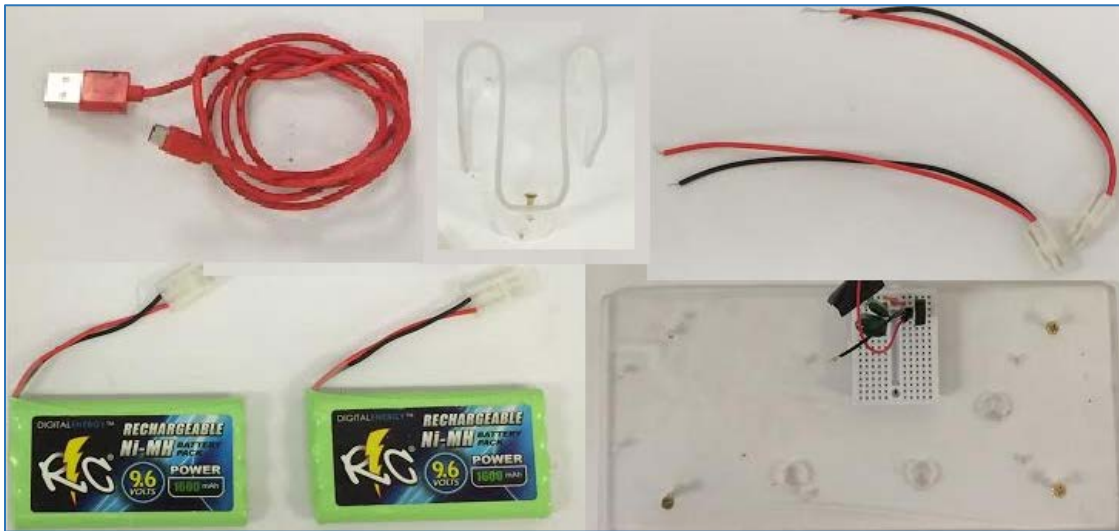
Figure 5. Cable, bracket, battery, platform, connector
