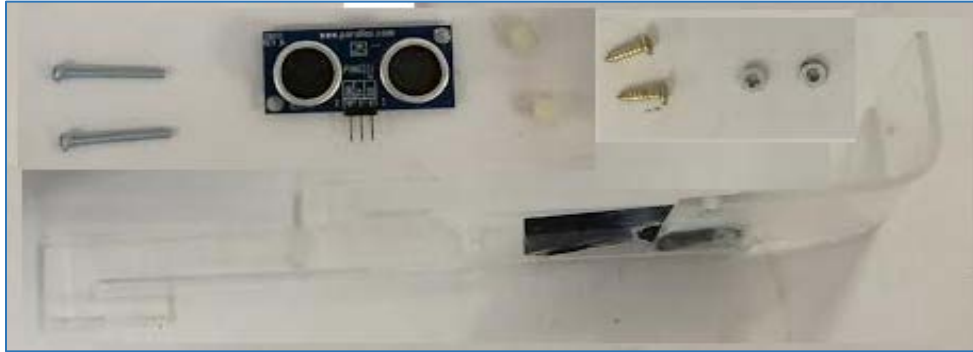
Figure 4. Screw (wood), ultrasound sensor, spacer, bolt, nut, plexiglas bracket
