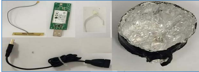
Figure 3. Antenna, Wi-Fi dongle, zip-tie, cable, Wi-Fi signal concentrator
