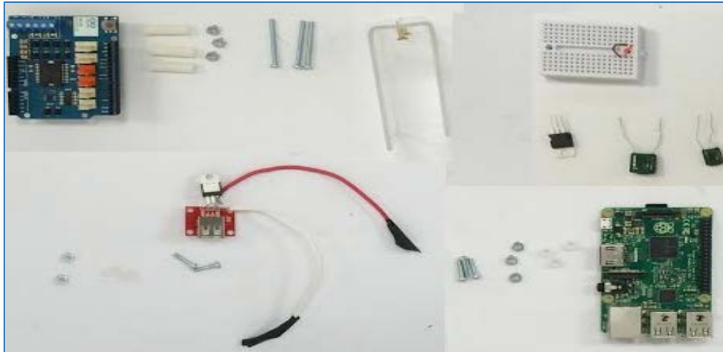
Figure 6. Motor shield, spacers, bolts, nuts, brackets, capacitors, 5V regulator, Raspberry Pi 2 B
