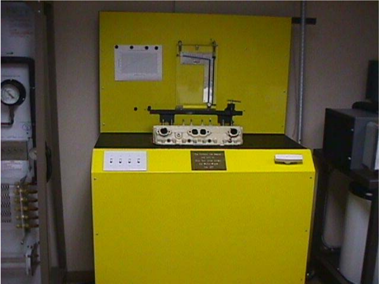
Figure 6. Completed Flow Bench
