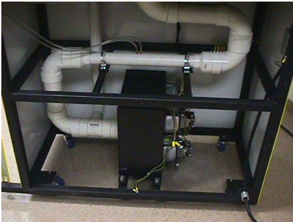
Figure 4. Flow Bench Frame – Actual
