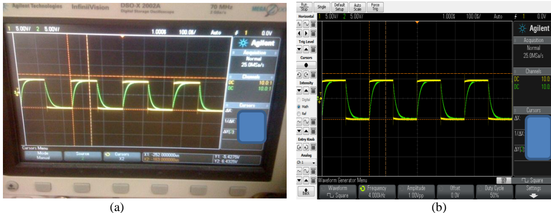
Figure 2a: Output of unknown RC circuit connected to physical Agilent Equipment. (b) Output of unknown RC circuit as seen through the virtual instrumentation connected to physical Agilent Equipment
