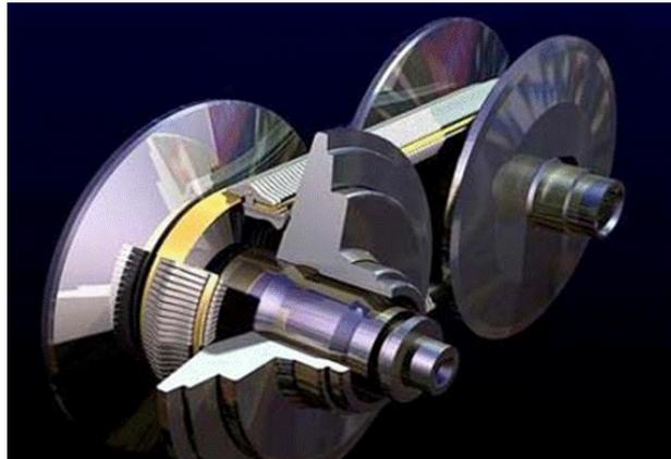
Figure 12: Variable Diameter Pulley CVT
