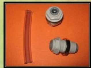
Push-locks with new flexible tubing
