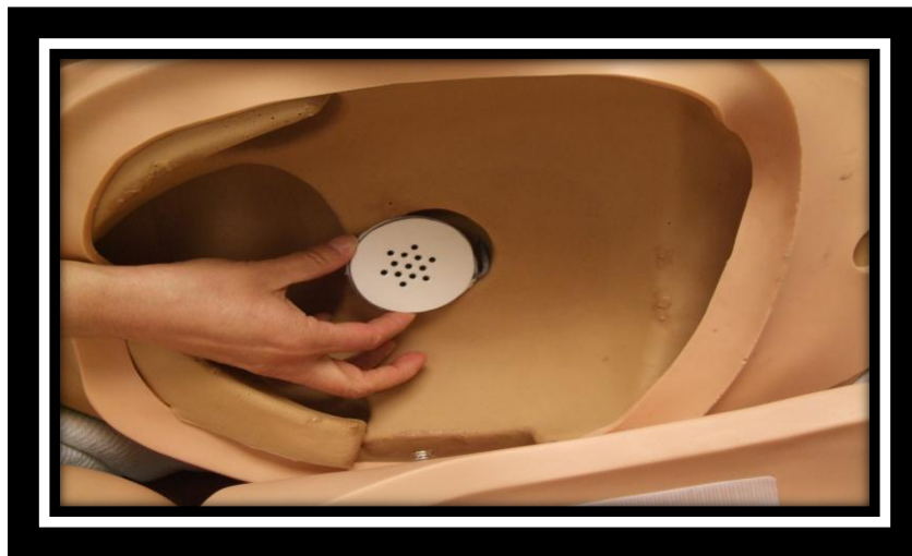
[Report] Figure 1: Fetal microphone in the abdominal foam of the manikin Noelle after the redesign.
