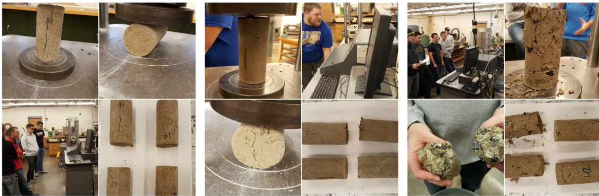
Figure 2: Different groups conducting compressive and tensile strength tests on Green Concrete samples
