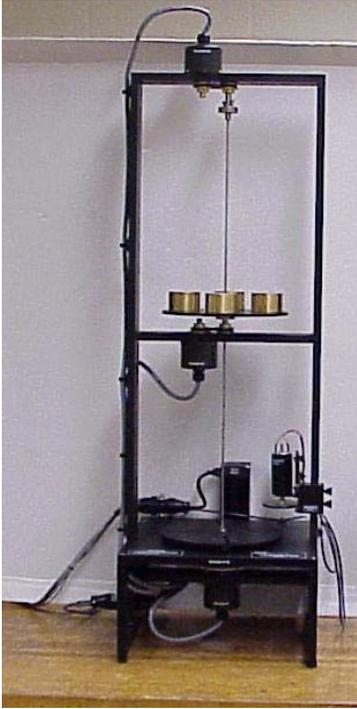
An unrestrained torsional mechanical system
