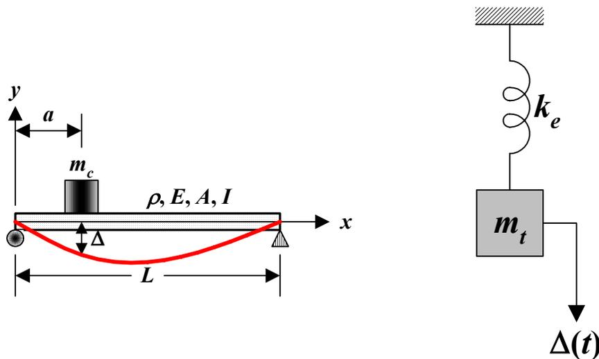
The problem is related to one of the prerequisites of the course: ME 33000: Mechanics of Materials. In order to find the equivalent spring constant and mass, students will need the results of beam deflection due to an equivalent concentrated force. Such a beam deflection may be obtained from a conventional Mechanics of Materials textbook. To demonstrate that background knowledge from Mechanics of Materials is needed, students are asked to solve this problem through the following steps:
