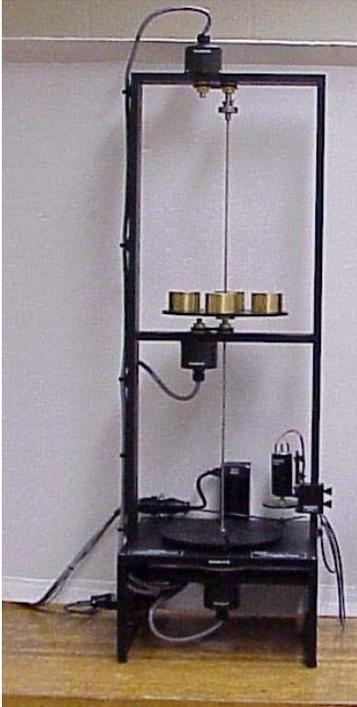
An unrestrained torsional mechanical system
