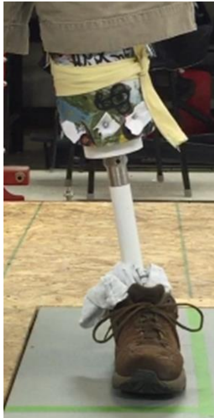
Figure 2: Preliminary prosthetic limb fitted to client's stump on force platform.
