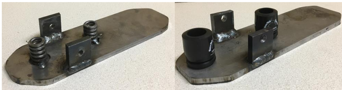
Figure 3: Base support with hinge supports and metal springs (left) and rubber springs (right)
