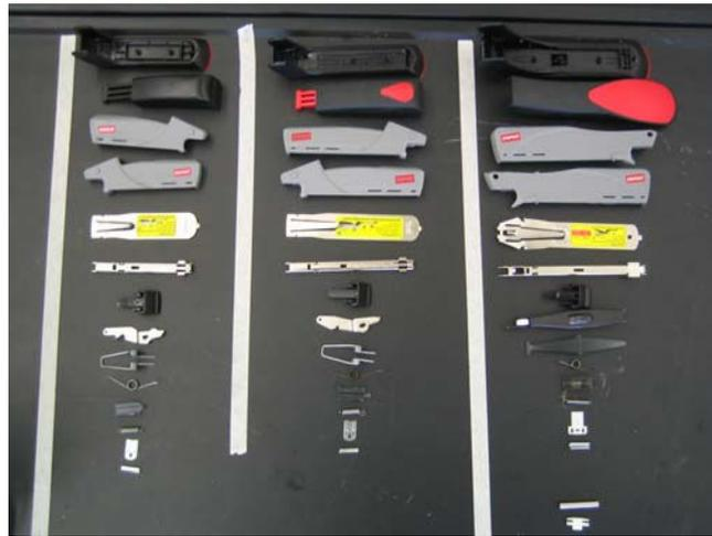
Figure 3. Three Stapler® One-Touch Staplers dissected to the component level.
