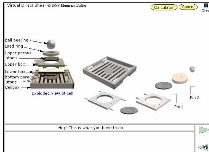
Figure 4 Parts of the cell a direct shear test that the student will set up using drag and drop interactions.
