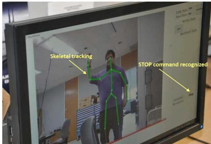
Figure 7 – (top) the Kinect depth sensing camera (retrieved from liliputing.com). (bottom) The OAR software interface showing skeletal tracking and the recognized STOP command gesture.
