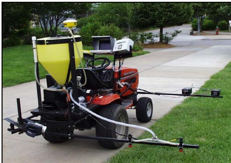
**Figure 2.** Weed detection system with variable rate applicator.
