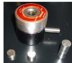
Figure 6. Pellet die for lab pelletization.
