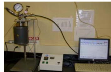
Figure 5. Parr Instruments, Inc., pressure vessel equipped with electronic controller and personal computer.
