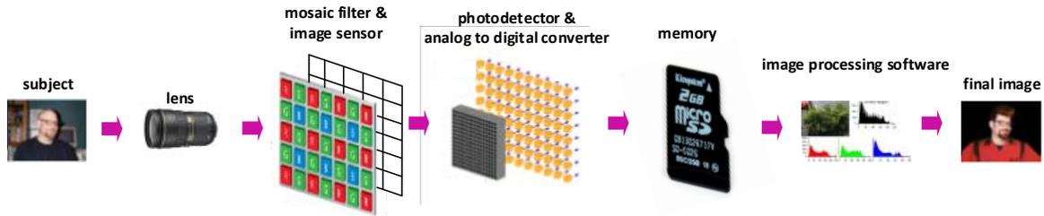
**Figure 3. An end to end process of how camera turns light into a processed digital image**
