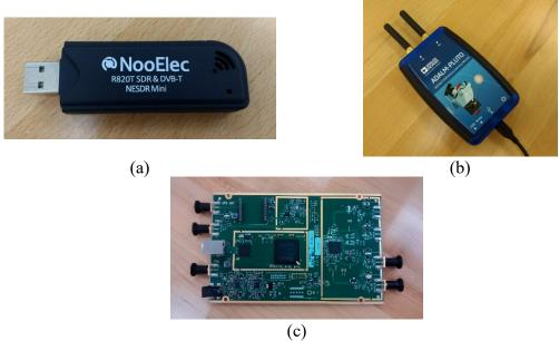
Figure 1: Software-defined radio devices. Commonly used SDR platforms used in engineering education include the RTL-SDR (panel (a), receive only, \$20), ADALM PLUTO (panel (b), transmit and receive, \$150), and ETTUS USRP B200 (panel (c), transmit and receive, \$750)
