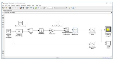
Figure 6: Simulink model for simulating passband FM waveforms
