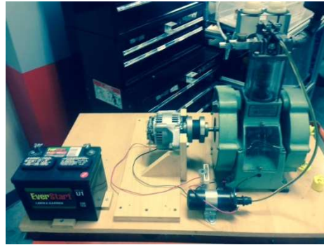
Figure 1. Ethanol Engine, DC Alternator, and Battery Load
