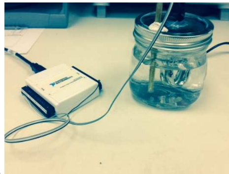
Figure 2. Joule Heating Experimental Set-up
